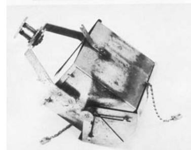
the spring-loaded scoops which spring shut, trapping a small sample of sediment. The sampler is then pulled to the surface, and the sample collected into a bucket or sample bag.
